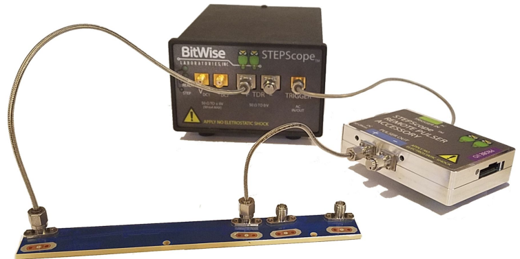
The STEPSCOPE™ Remote Pulser Accessory is used in conjunction with a STEPSCOPE™ analyzer (STEPSCOPEA) to make Insertion loss (S21) measurements
