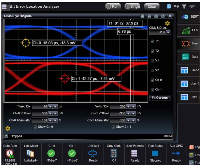
Quasi-Eye Diagram of Each Input Channel
