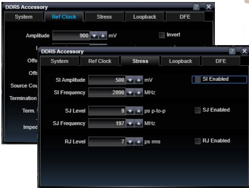
User interface to DDR5 Stress Accessory features is provided by the host analyzer.
